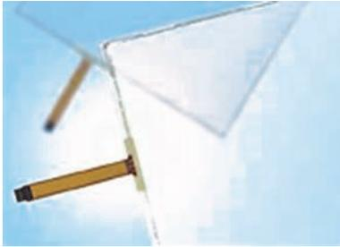
Known for innovative technology and products, 3M Touch Systems has leveraged decades of capacitive technology experience to create the MicroTouch™ SCT3250EX Capacitive touchscreens (formerly called ClearTek™ II Capacitive Touch System). MicroTouch Capacitive sensors have enhanced light transmission, with a very fast response to even the most gentle of touches.
